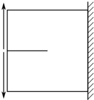
FIGURE – Opening crack.
