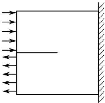
FIGURE – In plane shear crack.
